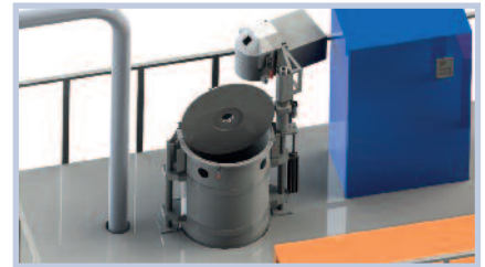
Easy change of alloy and atomisation nozzle for powder production in a wide range of particle sizes
